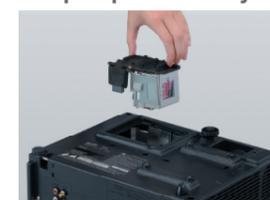
You can exchange the lamp easily and safely even when the projector is mounted on the ceiling or in another high location.
